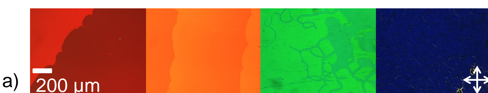
Figure 2 – polarized microscopy images of cholesteric mixtures of varying pitch, (b) schematic of planar aligned cholesteric liquid crystal cell reflecting light incident on the surface
