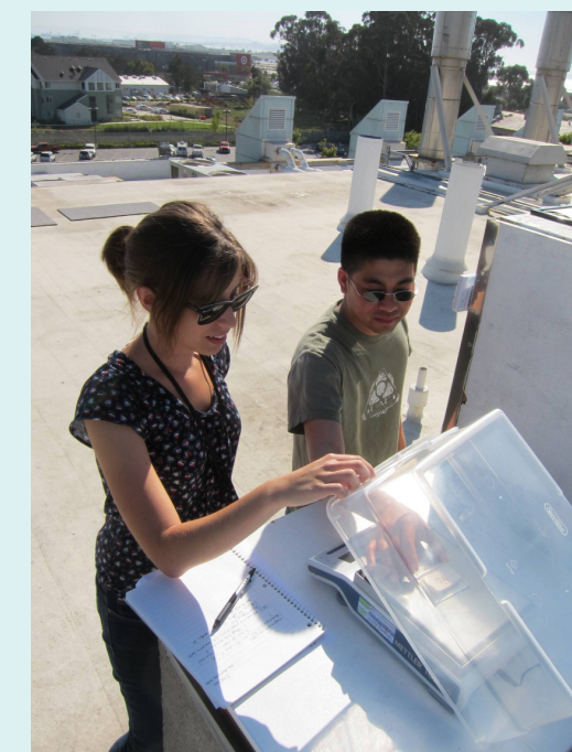
Technicians Laure Vallot and Matt Tom Conduct Sponge Drying Experiment with Solar Dryer Cabinet; Researcher Becky Milczarek Removes a Tray from the Solar Dryer
