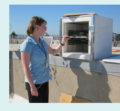
Technicians Laure Vallot and Matt Tom Conduct Sponge Drying Experiment with Solar Dryer Cabinet; Researcher Becky Milczarek Removes a Tray from the Solar Dryer
