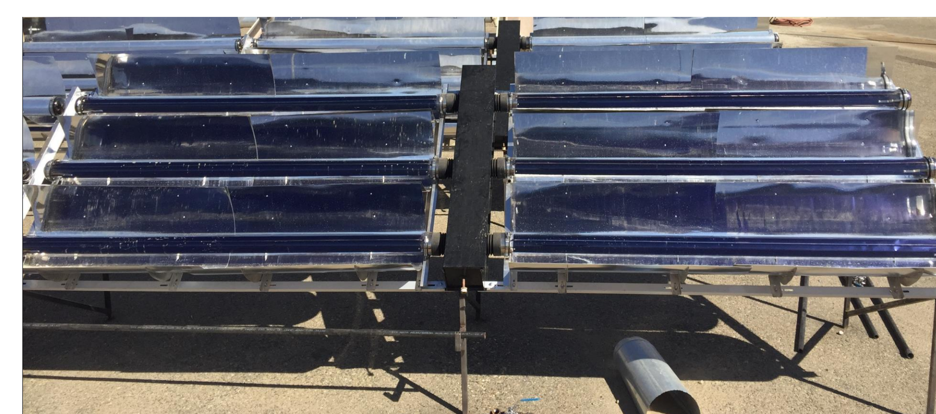
Fig. 5 - Fully Constructed East-West XCPC Prototype
