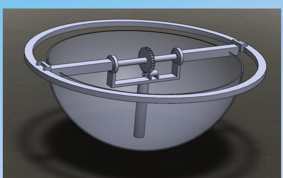
The latest model of the system. Each component is being built in small sections to be 3D printed for testing and calibration. Here you can see a motor that rotates the photovoltaic rod around the center axis. The outer circle will also rotate although this is not shown here
