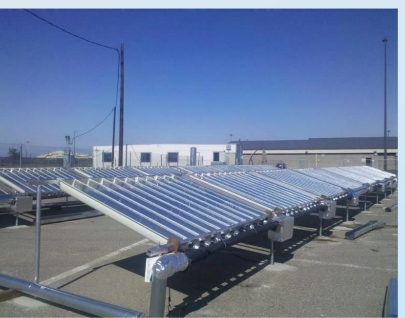
Solar Cooling successfully demonstrated using XCPC powered double effect absorption chiller for 4 seasons at UC Solar test facility in Merced.
